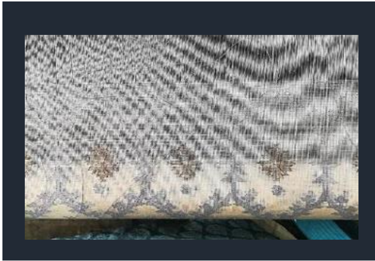
A saree with modern Jamdani design getting weaved on the loom
